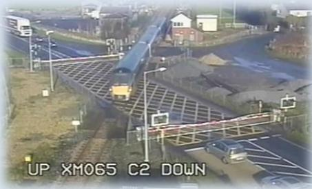
At approximately 11:10:56 hrs, the 09:45 hrs passenger service from Westport to Heuston (Train A805) triggered the initiation for Level Crossing XM065 (a CCTV level crossing with lights and full barriers), which resulted in the road traffic lights flashing to indicate to road users that rail traffic was approaching. Two cars approached the level crossing from the Athlone direction, after this initiation had commenced, with one car stopping on the yellow box area (Car 1),
