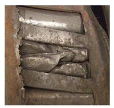
Photo 4 – Fractured Roller
