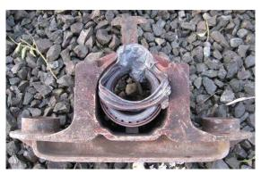
Photo 2 – Failed Bearing & Axlebox
