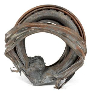
Photo 3 – Failed Bearing
