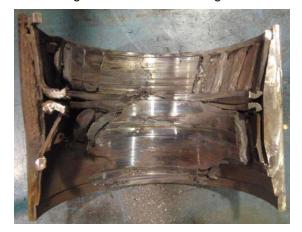
Figure 7 - Bearing cup raceways
