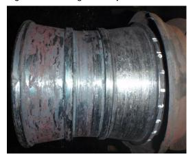
Figure 6 - Bearing cone raceways
