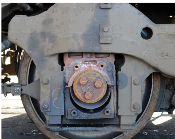
Figure 7 – Failed bearing on locomotive 233
