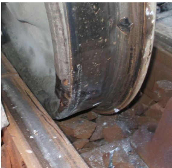
Photo 3 – Left derailed wheel
