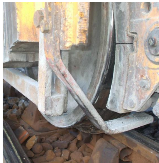
Photo 4 – Right derailed wheel
