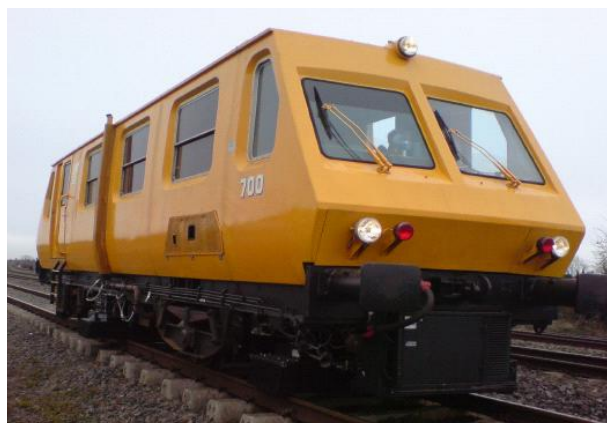
Photograph 7 – Track Recording Vehicle
