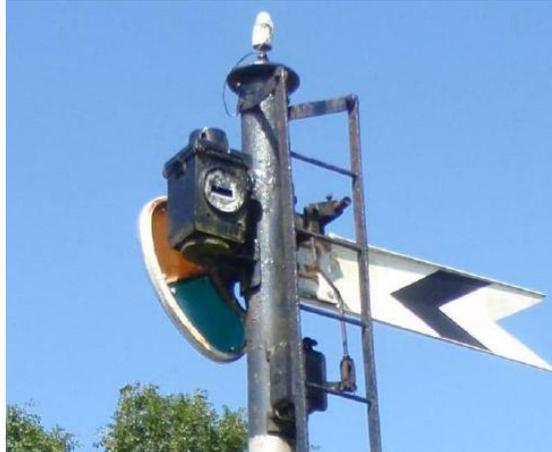
The semaphore signals display two aspects, ON and OFF. In between ON and OFF the signal is considered to be displaying an incorrect aspect and is called WRONG. For less than 5 degrees (°) above or below horizontal the signal is ON, from 5° to 30° below horizontal the signal is WRONG and from 30° to 55° the signal is displaying OFF, see Figure 3<sup>1</sup>.
