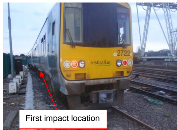
Figure 12 – First impact of tractor with train
