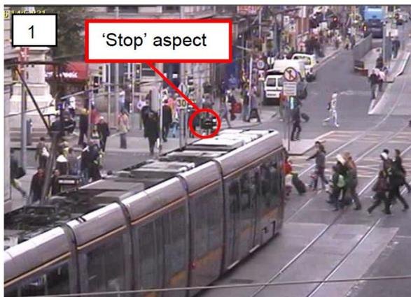
Tram stops at the stop line and remains at this point for 44 s. Tram aspect showing 'Stop'.
