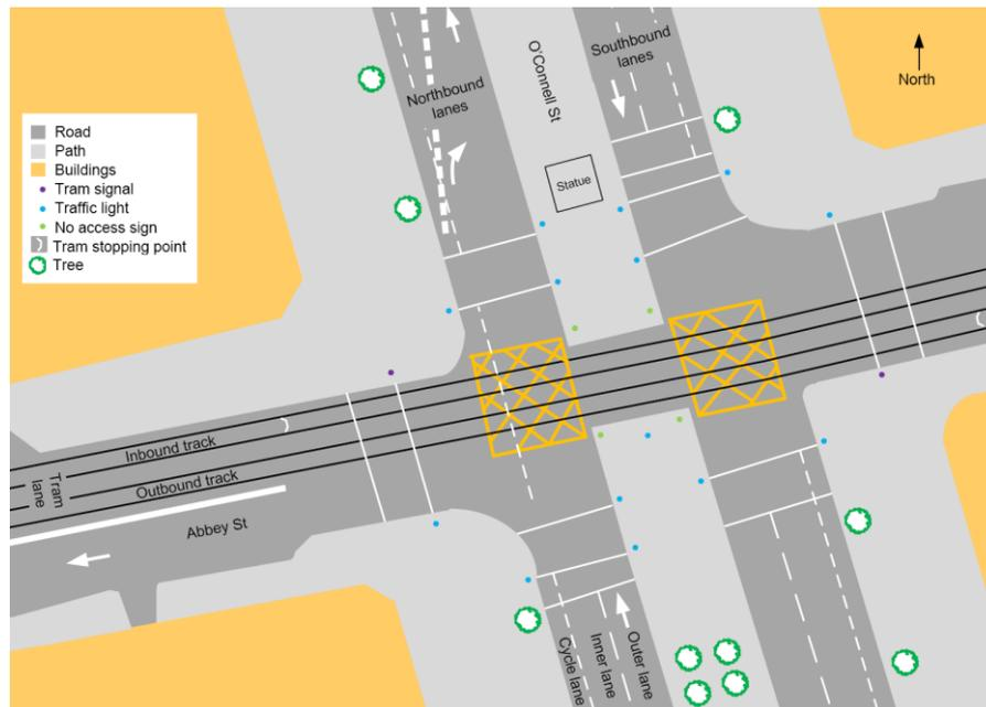
**Figure 2 – Junction Layout (not to scale, for illustration only)**
