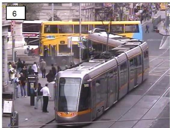
Tram derails and bus is pushed across the junction. Tram aspect remains at 'Stop'.
