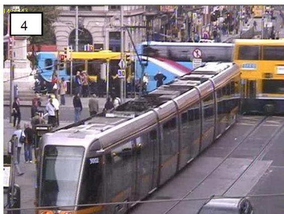
Bus enters the junction as the tram moves through the signal. Tram aspect remains at 'Stop'.
