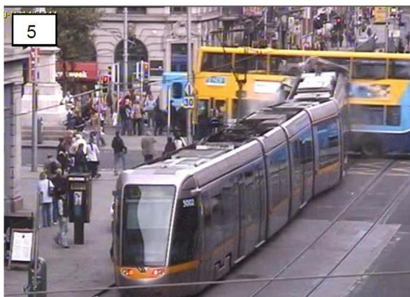
Tram impacts with the bus as it travels through the junction. Tram aspect remains at 'Stop'.
